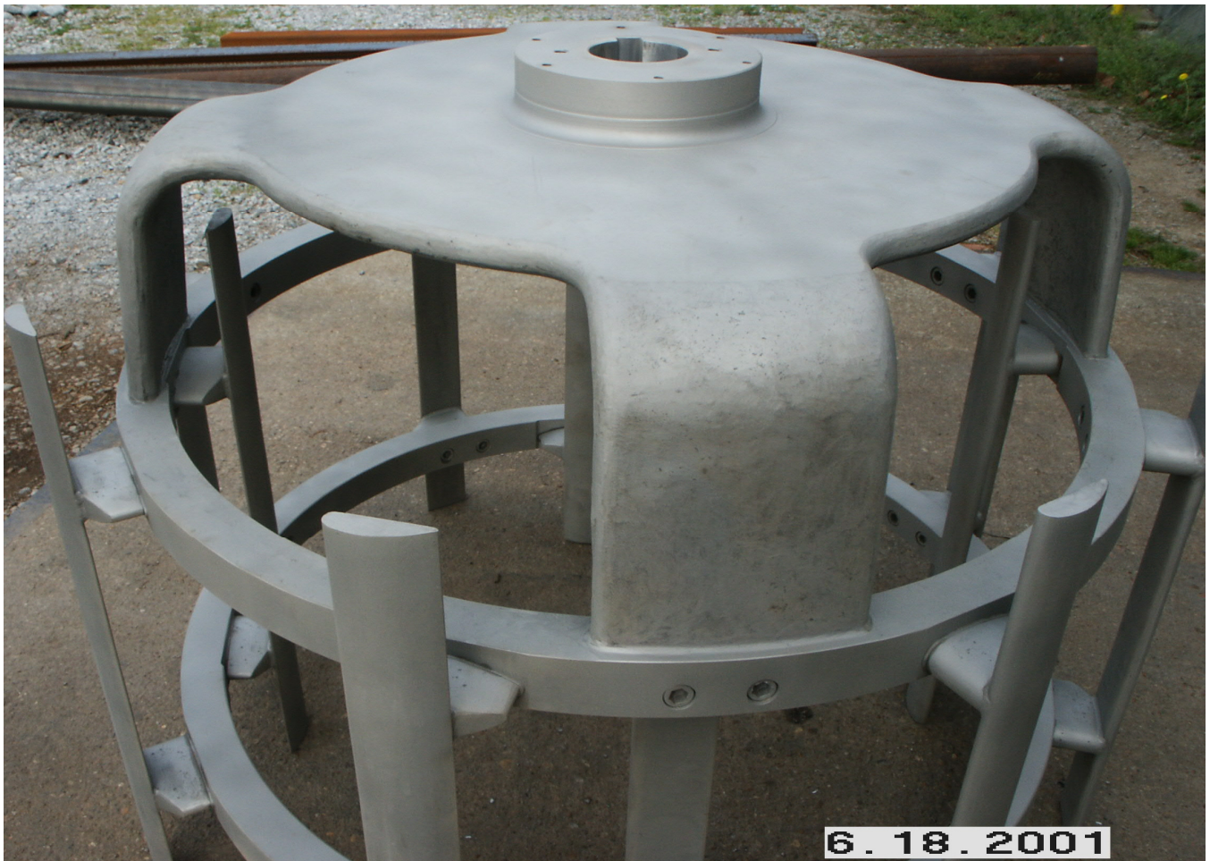
New Rotating assembly for Bird ( Voith ) Model 70 Centriscreen
