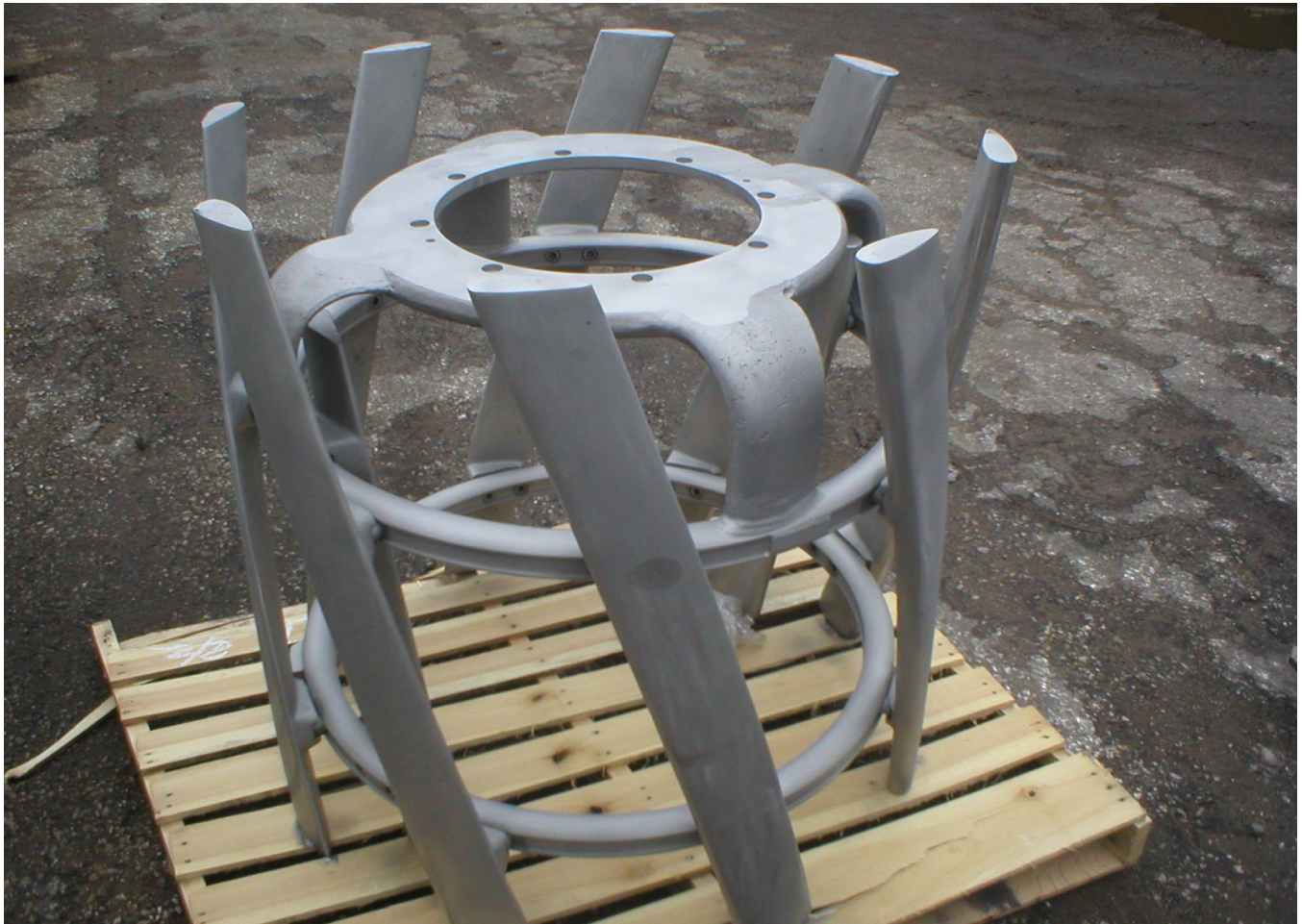
Rotating assembly for Voith Model 60 pressure screen
