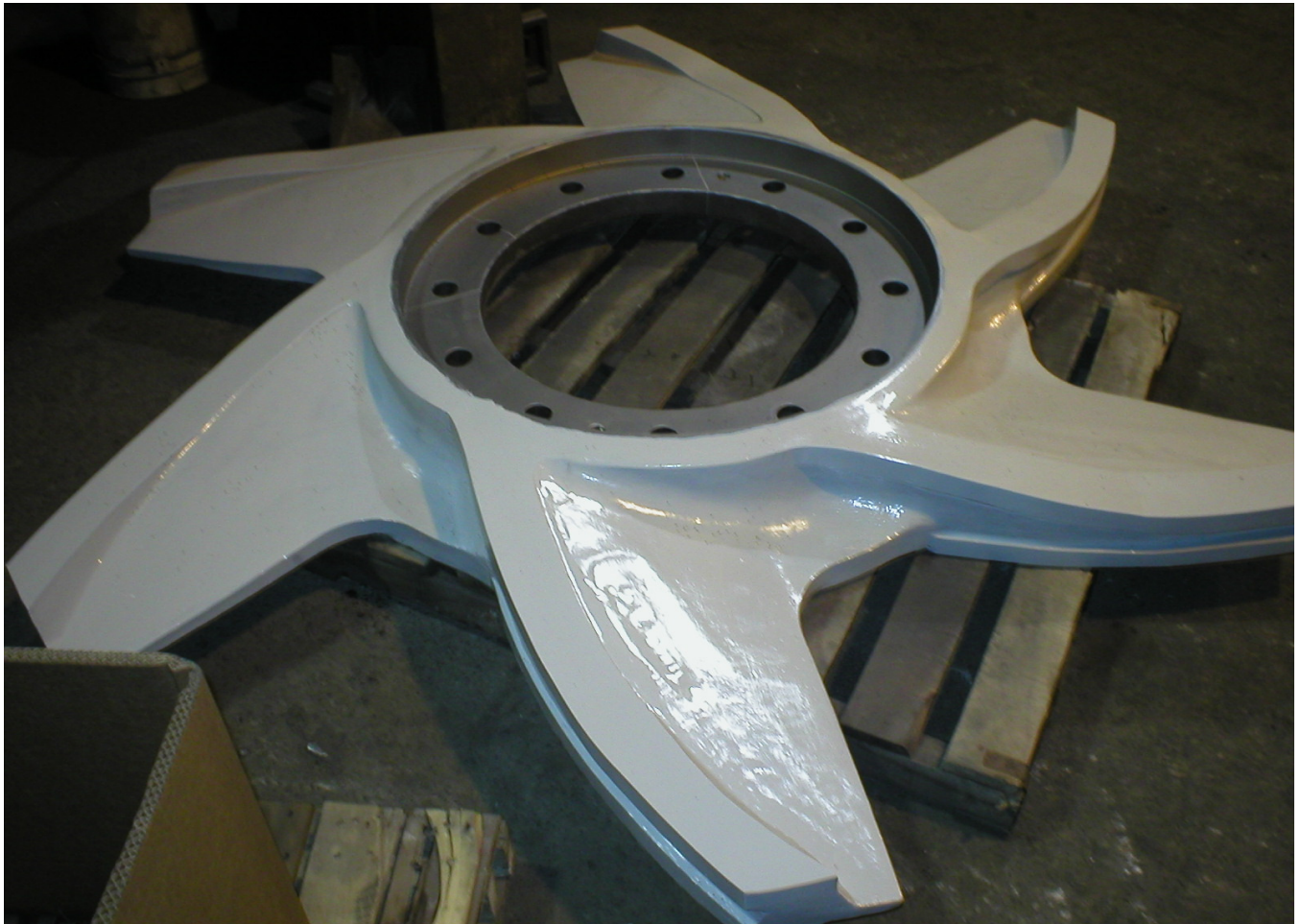
Rebuilt rotor for VSAP 60 300 ton Pulper
