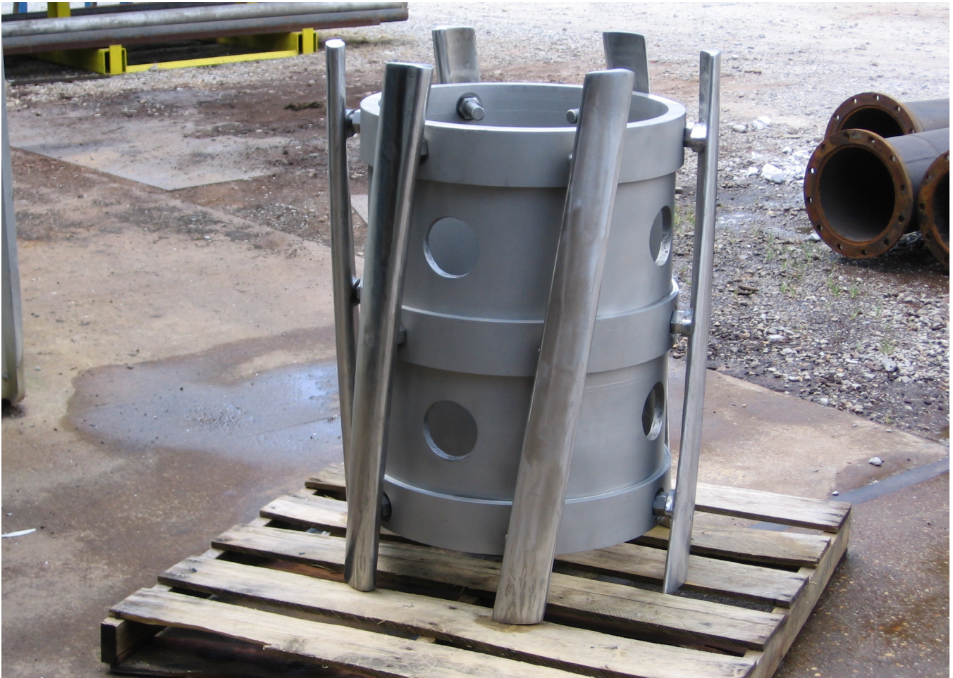
New Rotating Element and Foils for Black Clawson UV500 Pressure Screen
