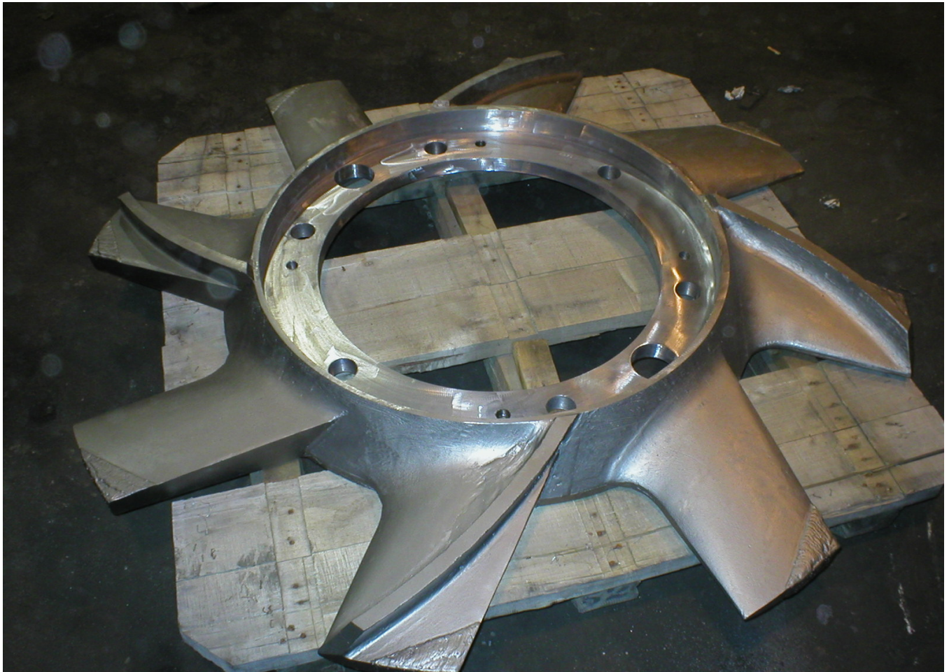
63" Rotor made to run with Black Clawson Mid-Con Turbine
