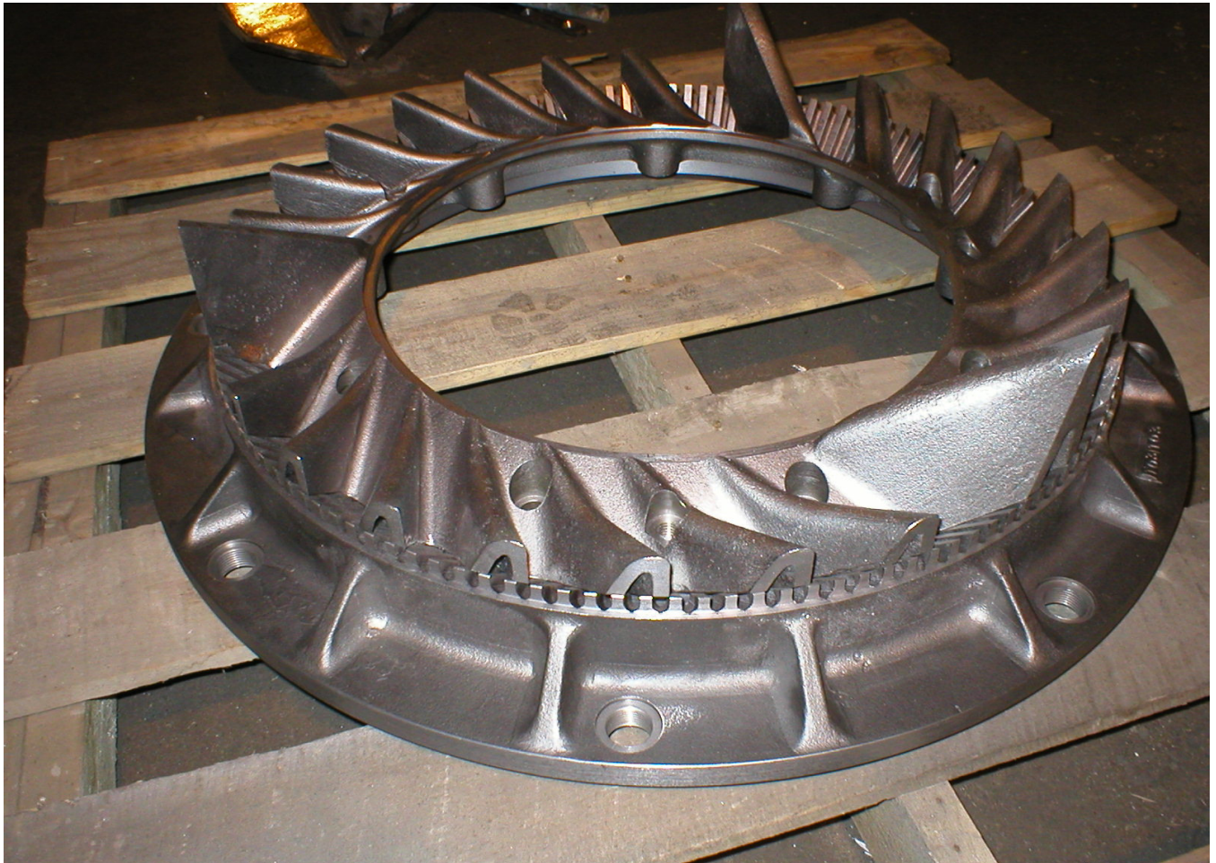
34" Slushmaker rotor and Defibering ring
